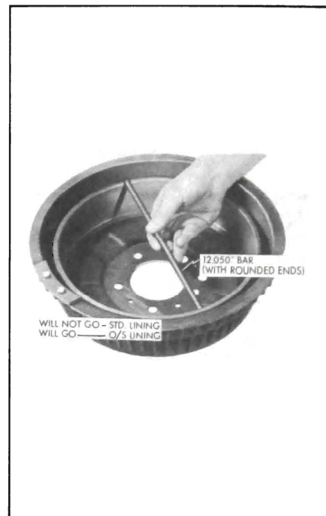
Figure 9-12—Measuring Brake Drum Size
