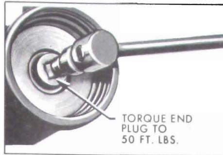
Figure 8-59—Torquing Rack-Piston Nut End Plug
