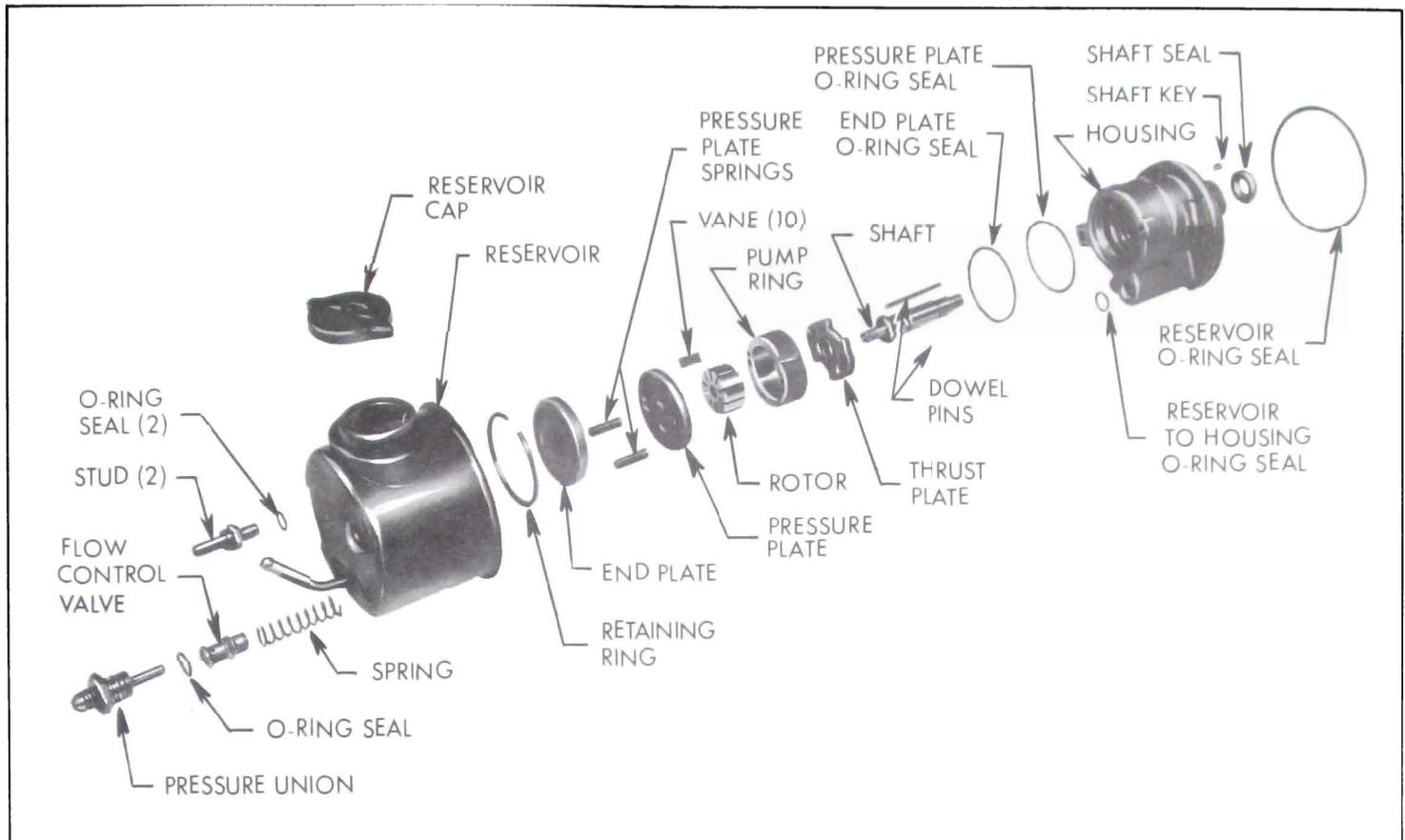
Figure 8-61—Exploded View of Oil Pump
