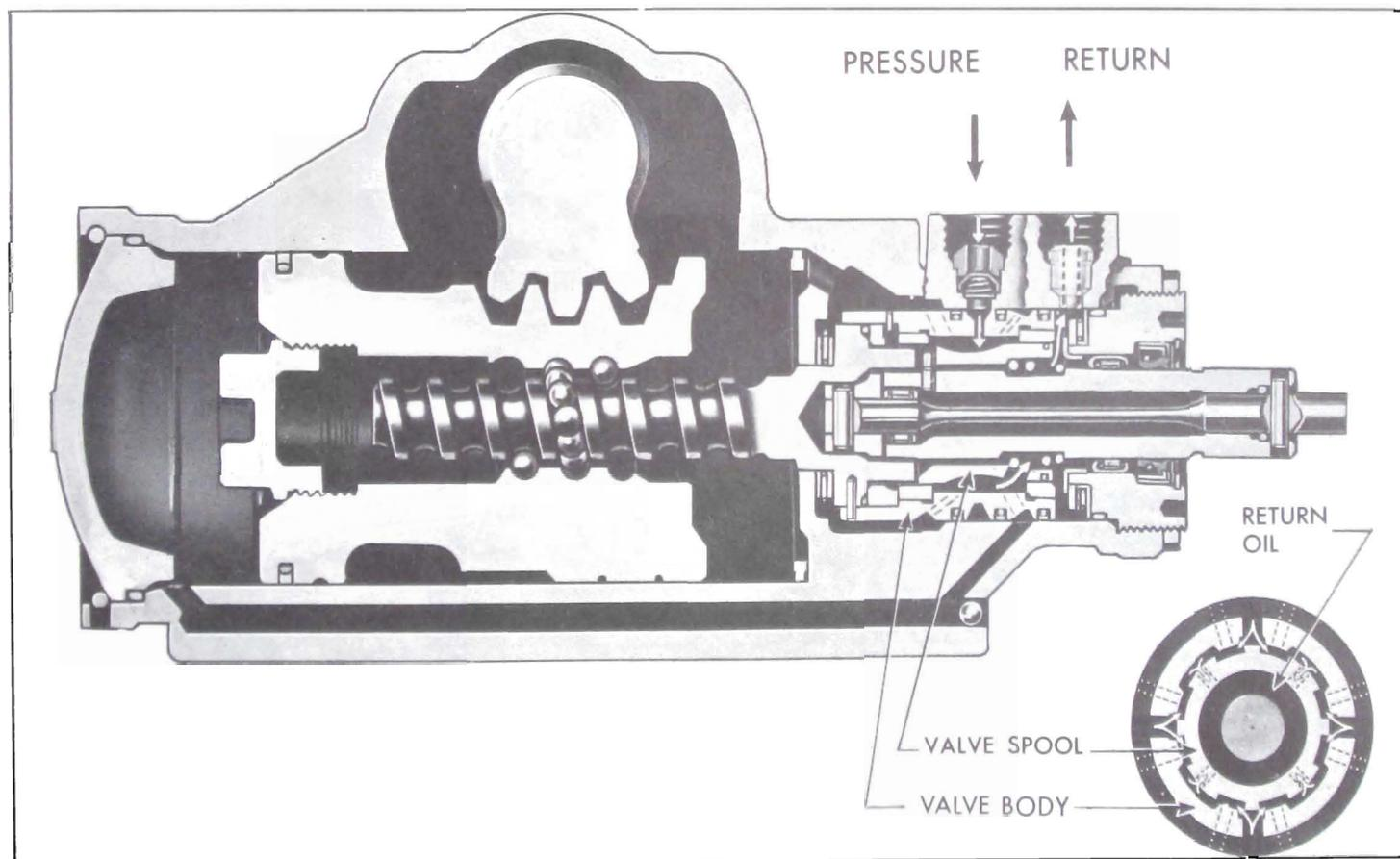
Figure 8-22—Oil Flow—Straight-Ahead
