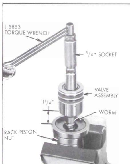
Figure 8-57—Checking Rack-Piston Nut Ball Preload
