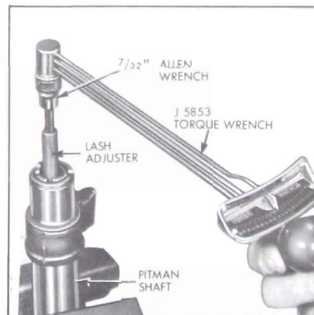
Figure 8-49—Checking Torque on Lash Adjuster
