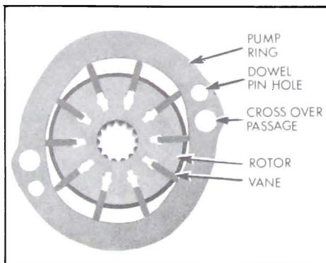
Figure 8-20—Pump Ring and Rotor
