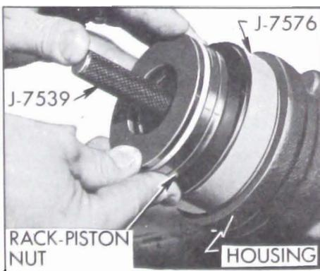
Figure 8-58—Installing Rack-Piston Nut
