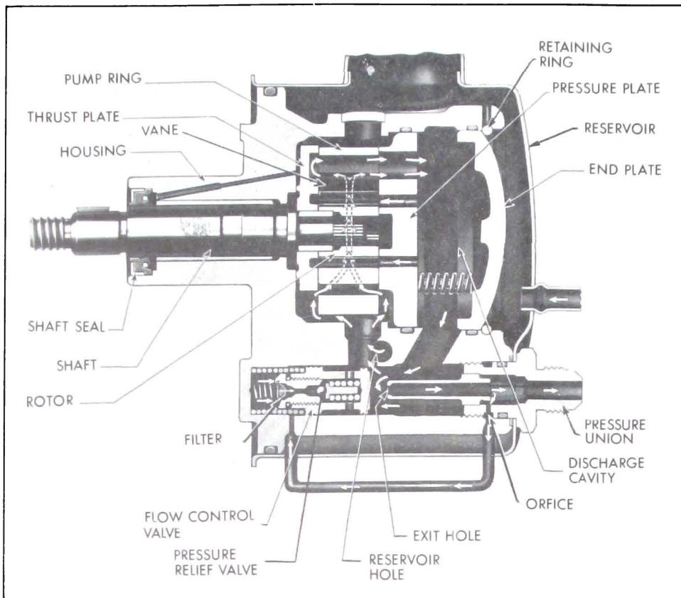
Figure 8-18—Oil Flow in Pump
