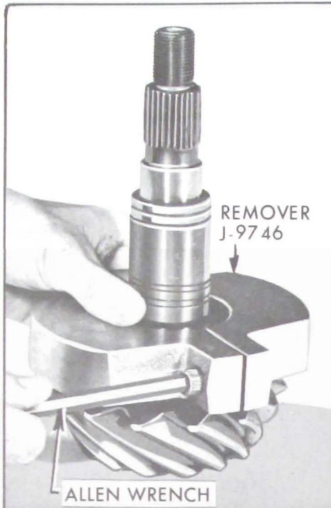
Fig. 6-62—Installing Pinion Bearing Remover
