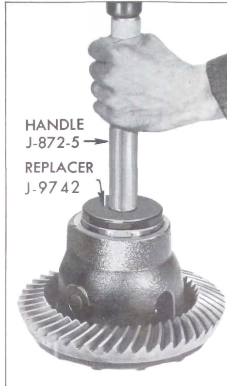
Fig. 6-75—Installing Differential Bearing Outer Race
