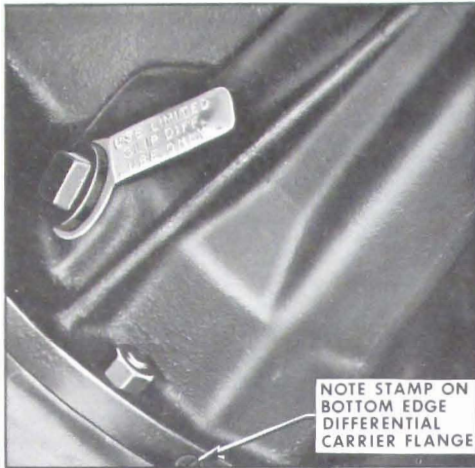
Figure 6-83—Identification of Positive Traction Differential Axle
