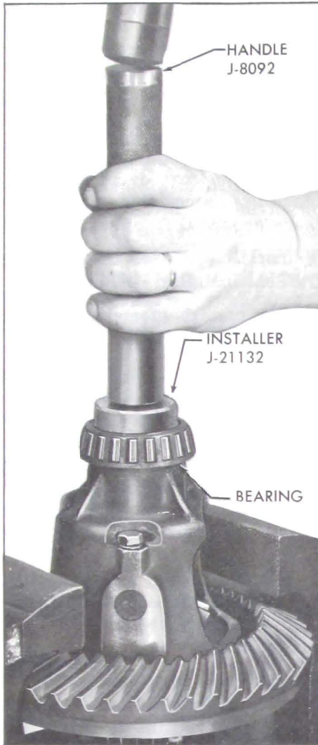
Fig. 6-30—Installing Differential Side Bearings
