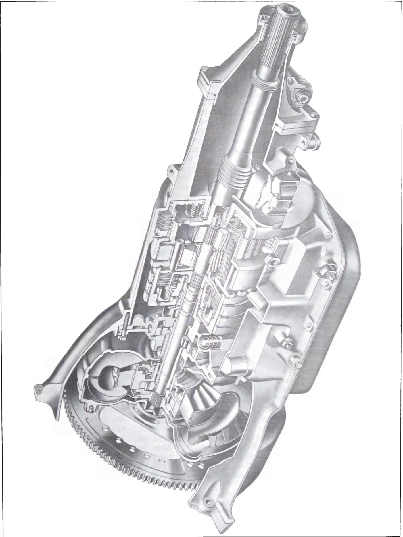
Figure 5-9—Cross Section of Transmission
