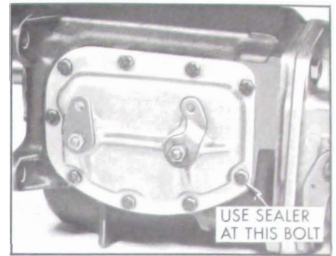
Figure 4-119—Transmission Side Cover Assembly
