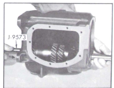
Figure 4-127—Removing Countergear with J-9573
