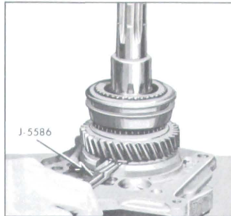
Figure 4-137—Installing Rear Bearing Retainer
