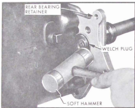
Figure 4-107—Installing Welch Plug
