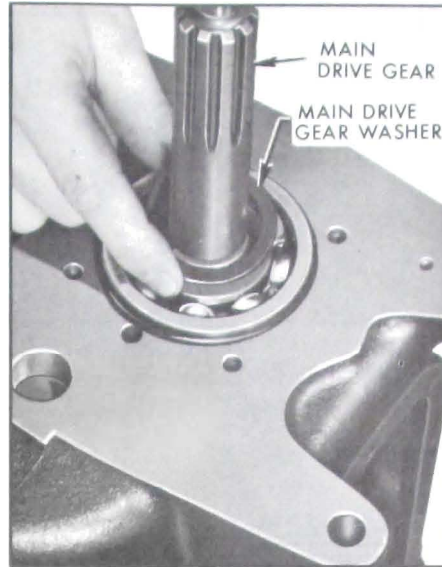
Figure 4-102—Main Drive Gear Washer Installation
