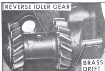
Figure 4-24—Idler Shaft Removal
