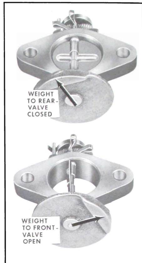
Figure 3-15—Manifold Heat Control Valve Positions - 401 and 425 Engines
