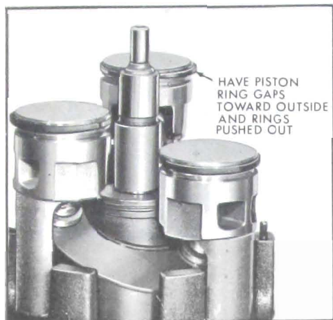
Figure 11-141—Pistons Positioned in "Stair Step" Arrangement
