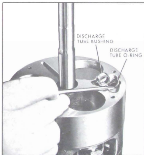
Figure 11-146—Installing Discharge Tube "O" Ring and Bushing
