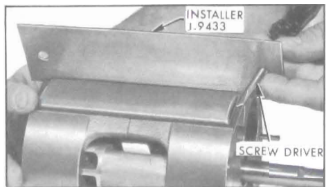
Figure 11-144—Removing Installer J-9433
