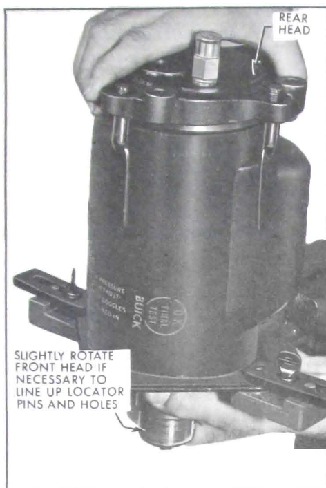
Figure 11-152—Installing Rear Head
