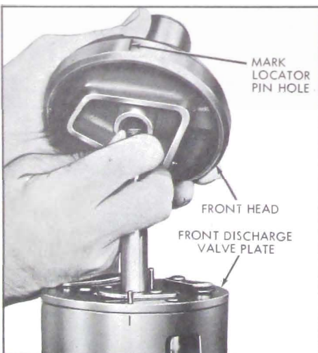
Figure 11-148—Installing Front Head on Cylinder Assembly
