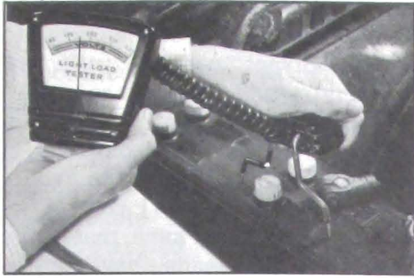
Figure 10-3—Light Load Test
