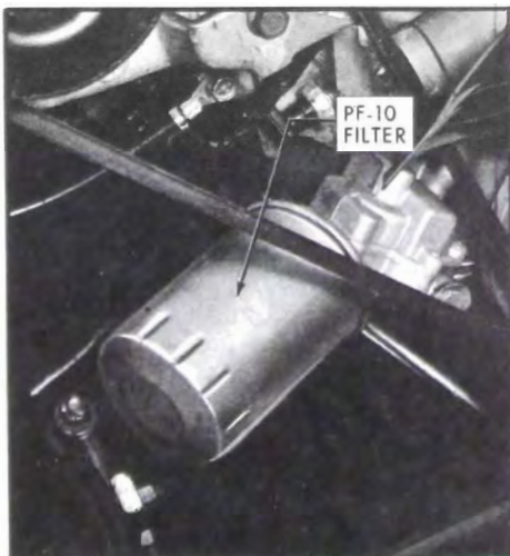
Figure 1-5—Oil Filter Installation
