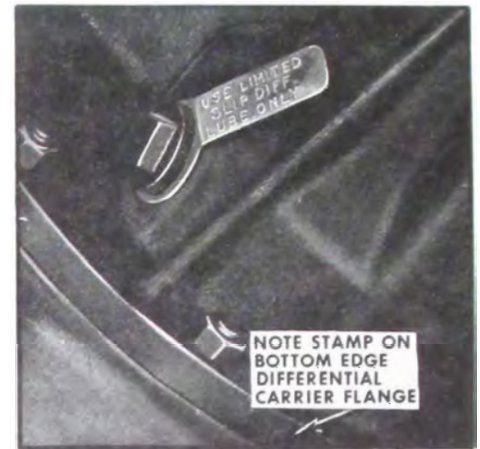
Figure 1-10—Identifying Positive Traction Differential
