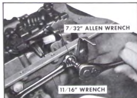
Figure 1-17—Backing Off Low Band Screw
