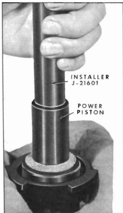
Figure 9-29—Installing Floating Control Valve Assembly
