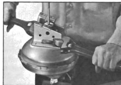
Figure 9-19—Power Brake Unit Positioned in a Vise
