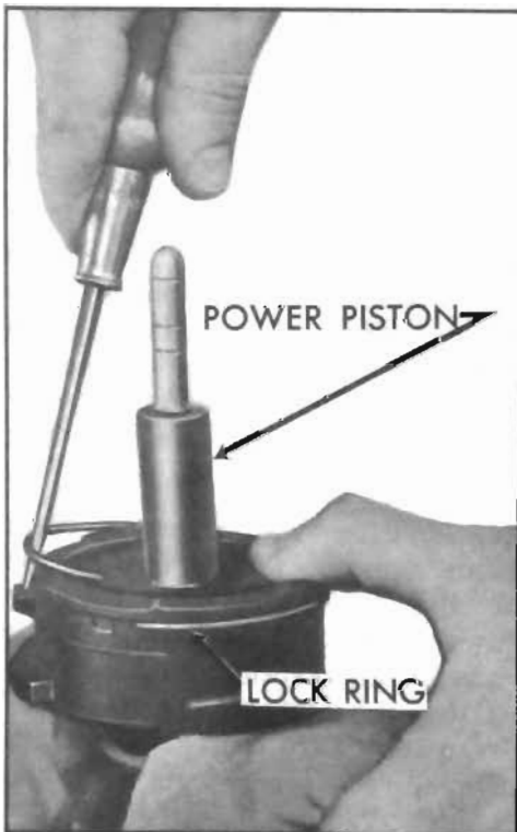
Figure 9-31—Installing Power Piston Lock Ring
