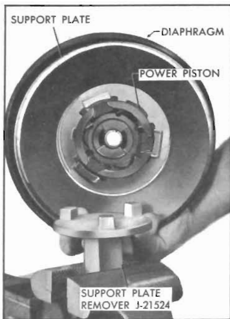
Figure 9-23—Positioning Support Plate Remover in a Vise
