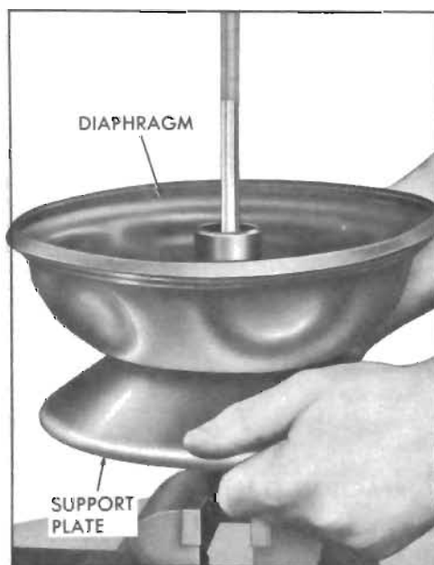
Figure 9-24—Positioning Power Piston on Support Plate Remover
