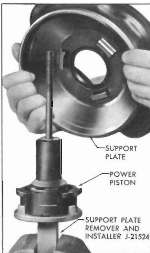
Figure 9-30—Installing Power Piston into Support Plate
