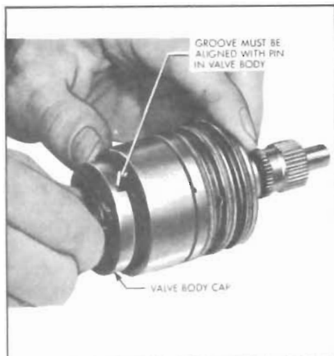
Figure 8-44—Assembling Stub Shaft, Torsion Bar and Cap Assembly in Valve Body
