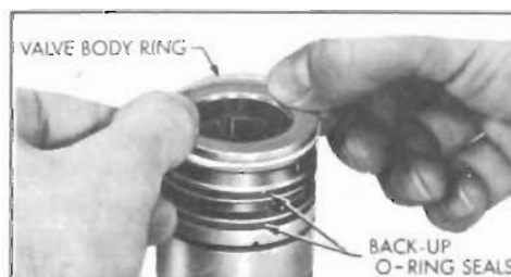
Figure 8-43—Installing Valve Body Rings
