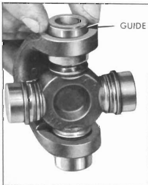
Figure 6-48—Installing Guide on U-Joint
