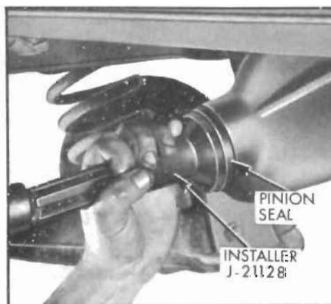
Figure 6-26—Installing Pinion Oil Seal
