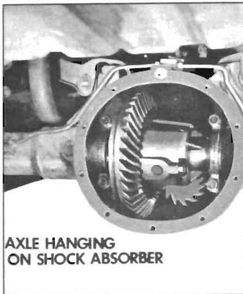
Figure 6-4—Rear Axle Assembly in Position for Repair
