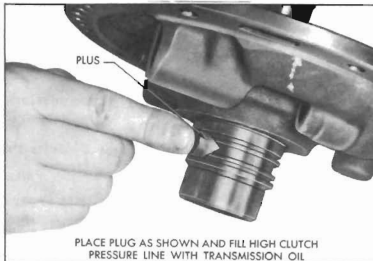
Figure 5-363—Checking Cross Leakage Between Pump Cover and stator shaft
