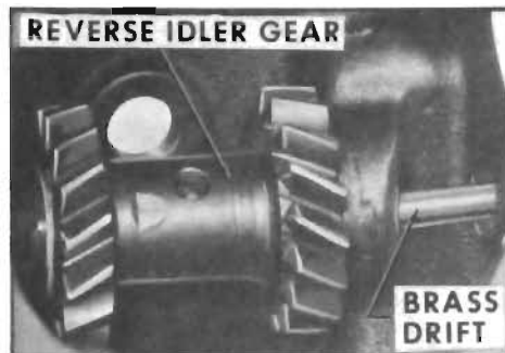
Figure 4-18—Idler Shaft Removal
