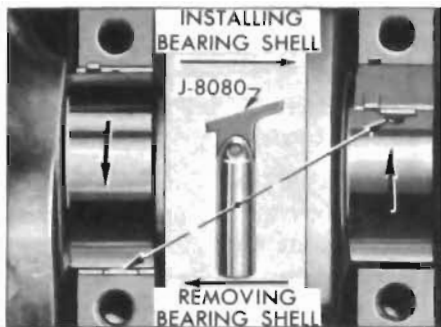
Figure 2-78—Removal and Installation of Crankshaft Bearing Upper Shell
