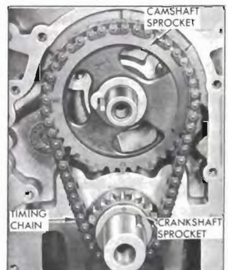
Figure 2-75—Installation Of Timing Chain and Sprocket
