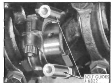
Figure 2-81—Connecting Rod Bolt Guides Installed
