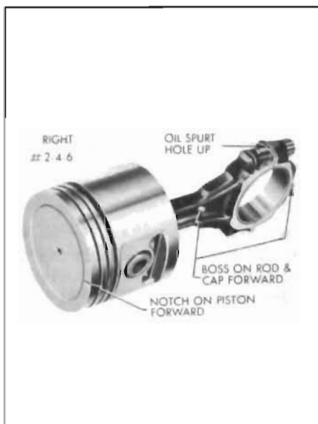
Figure 2-51—Piston and Connecting Rod have a groove or bevel cut around the inner edge on one side. The top compression ring is installed
