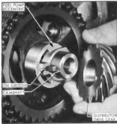
Figure 2-76—Fuel Pump and Distributor Drive Gear Installation
