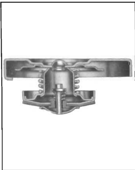
Figure 2-55—Engine Radiator Cap Cross Section
