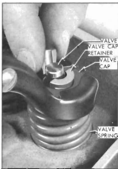
Figure 2-19—Removing Valve Cap Retainers
