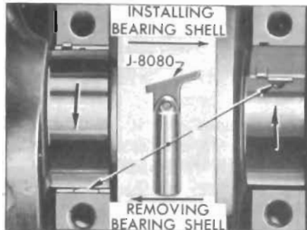
Figure 2-31—Removing and Installing Crankshaft Bearing Upper Shell
