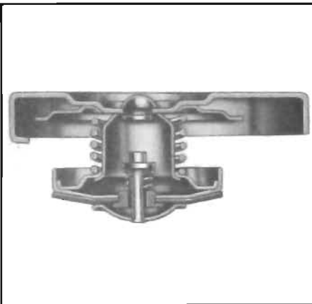
Figure 2-8—Engine Radiator Cap Cross Section
