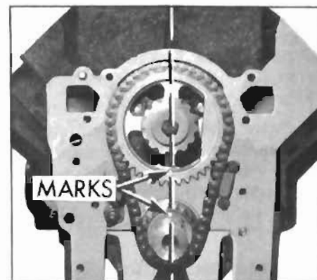
Figure 2-28—Proper Installation of V-6 Timing Chain and Sprocket
