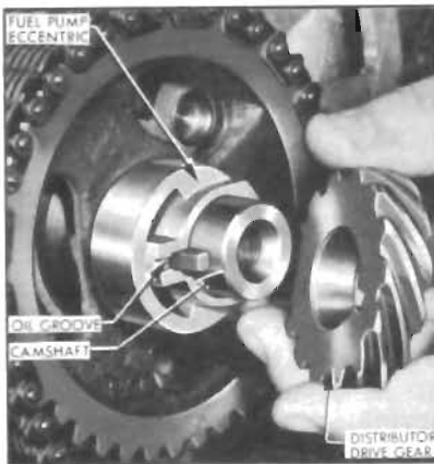
Figure 2-29—Fuel Pump and Distributor Drive Gear Installation
