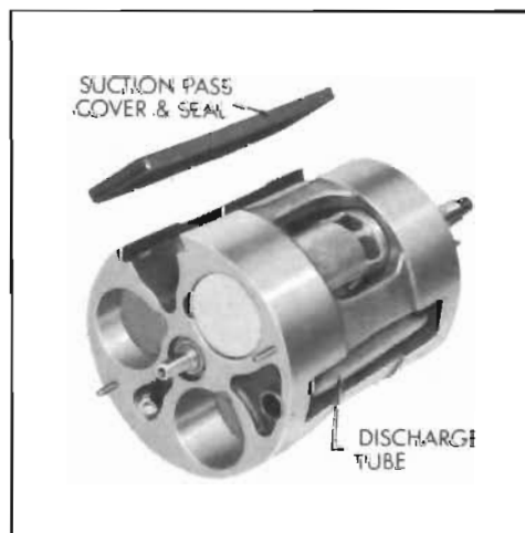
Figure 11-34—Suction Passage and Discharge Tube
