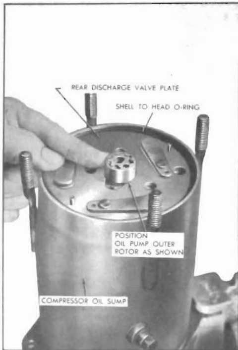
Figure 11-103—Positioning Oil Pump Outer Rotor
