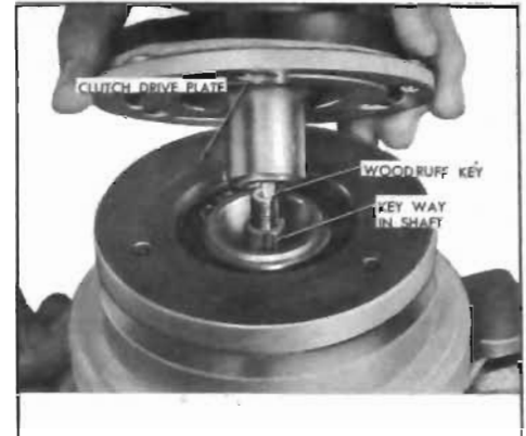
Figure 11-59—Positioning Clutch Drive Plate on Shaft
