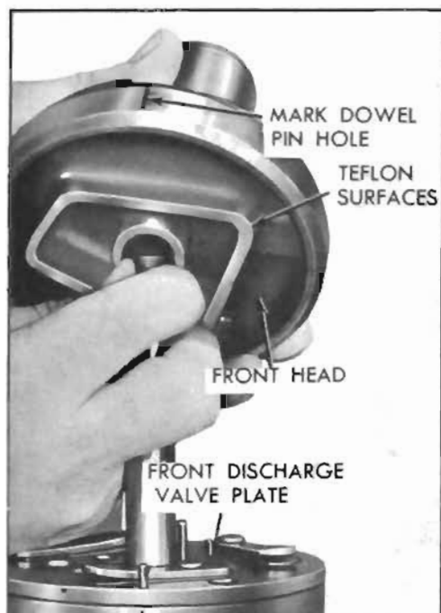
Figure 11-100—Placing Front Head on Cylinder Assembly
