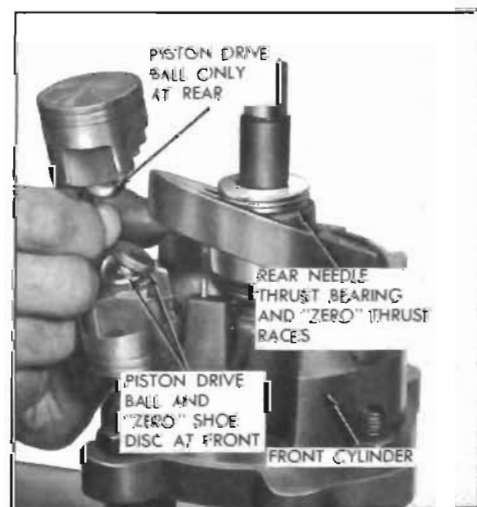
Figure 11-83—Installing Piston into Cylinder Half
