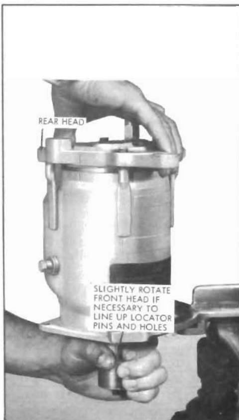
Figure 11-104—Installing Rear Head
