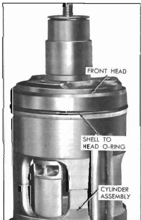
Figure 11-101—Shell to Head O-Ring Installation
