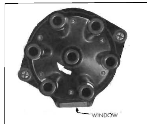
Figure 10-44—Installing Spark Plug Wires in Cap (V-6 Engine)
