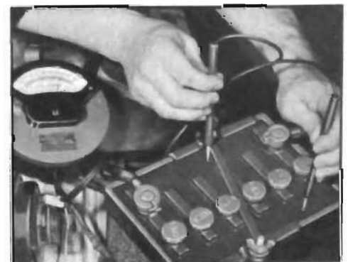
Figure 10-3—Light Load Test
