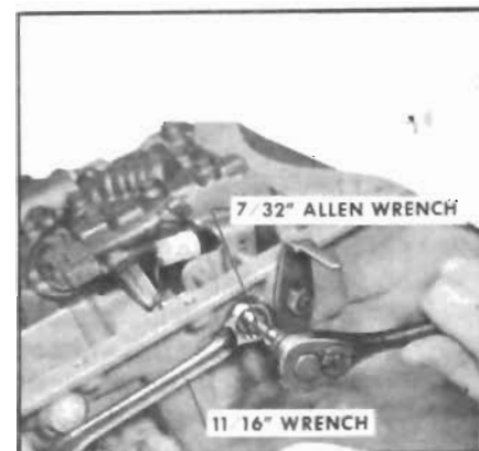
Figure 1-12—Torquing Low Band Screw
