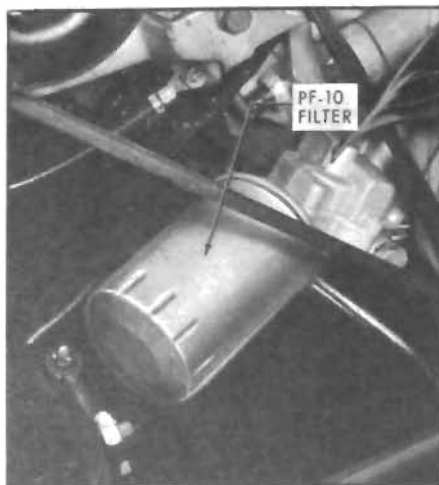
Figure 1-4—Oil Filter Installation
