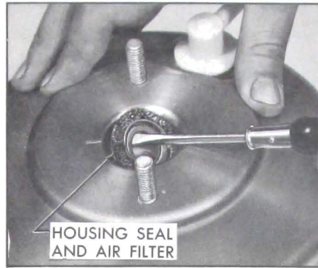
Figure 9-23—Removing Housing Air Cleaner and Guide Seal
