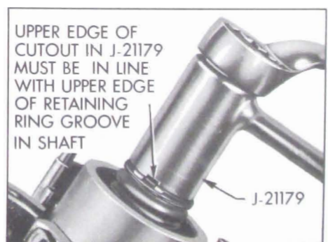
Figure 8-93—Compressing Preload
