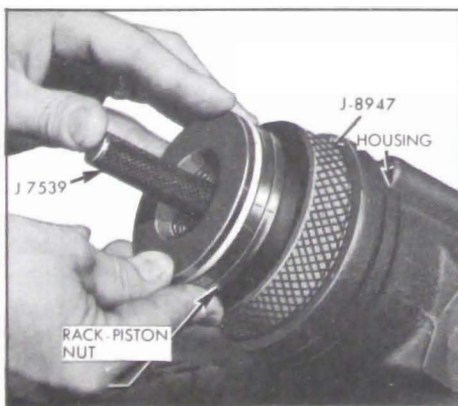
Figure 8-58—Installing Rack-Piston Nut
