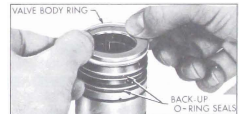
Figure 8-43—Installing Valve Body Rings
