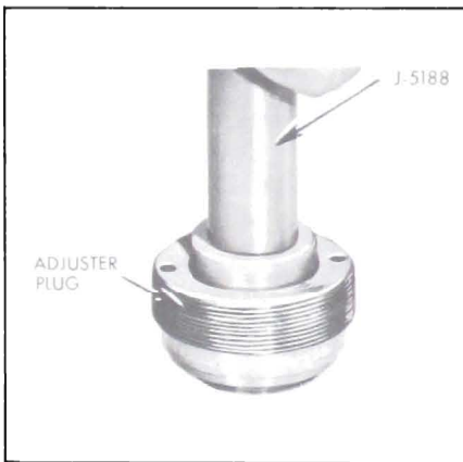
Figure 8-38—Installing Stub Shaft Seal
