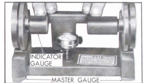
Figure 6-20—Zeroing Pinion Setting Gauge
