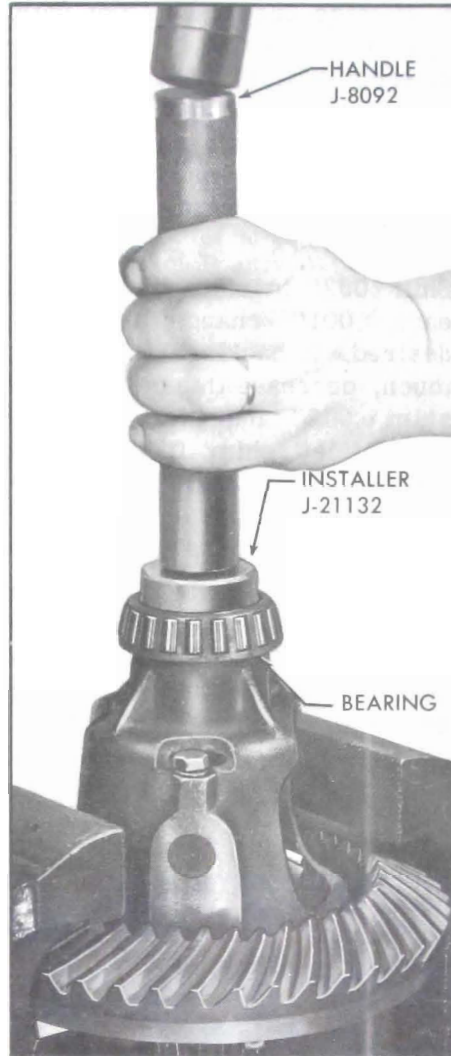
Figure 6-30—Installing Differential Side Bearings
