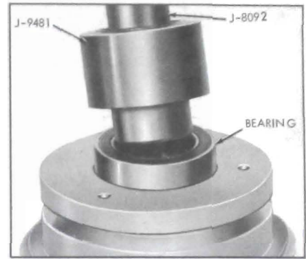
Figure 11-67—Installing Bearing into Pulley Assembly
