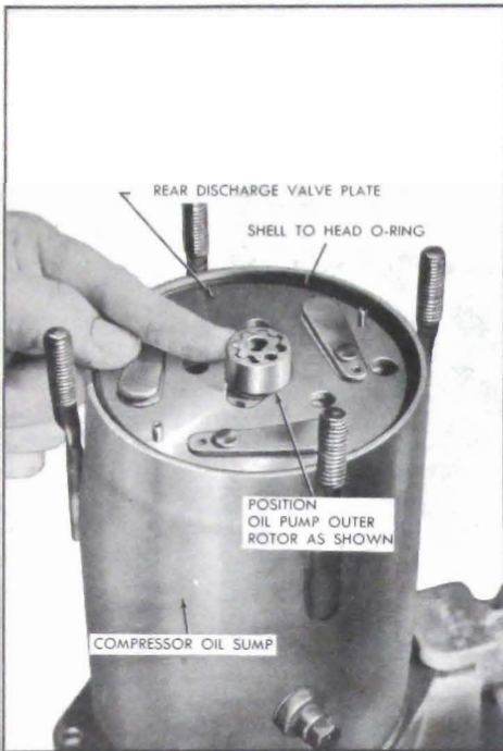
Figure 11-103—Positioning Oil Pump Outer Rotor
