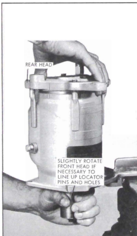
Figure 11-104—Installing Rear Head
