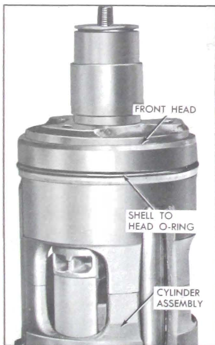
Figure 11-101—Shell to Head O-Ring Installation
