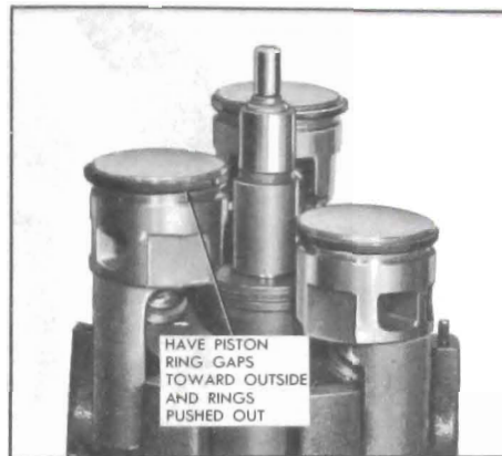
Figure 11-95—Pistons Position In "Stair-Step" Arrangement
