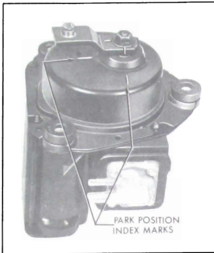
Figure 10-73—Park Position of Crank Arm
