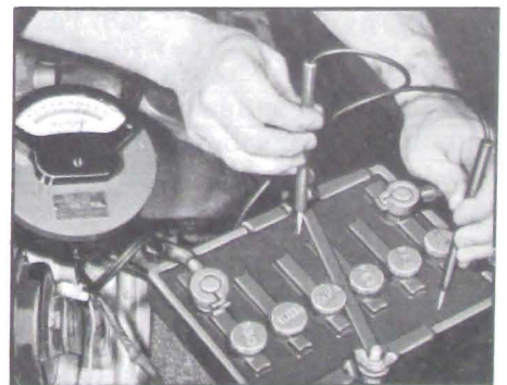
Figure 10-3—Light Load Test
