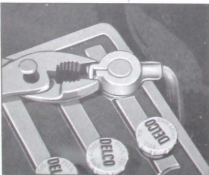
Figure 10-6—Removing Battery Cable
