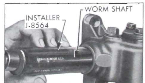
Figure 8-12—Installing Worm Shaft Seal
