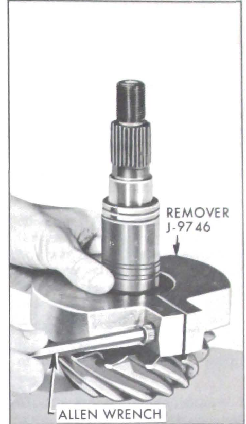
Figure 6-19—Installing Pinion Bearing Remover
