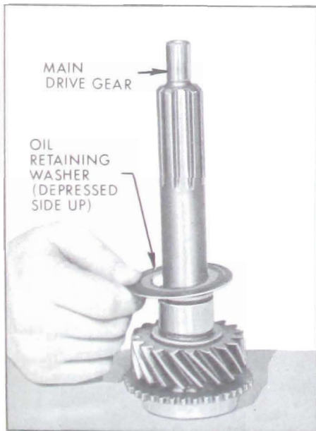
Figure 4-100—Installing Oil Retaining Washer
