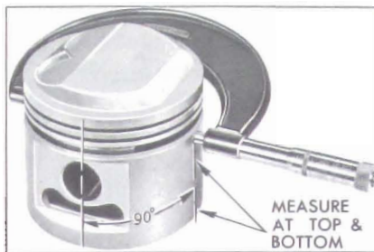
Figure 2-42—Measuring Piston with Micrometer
