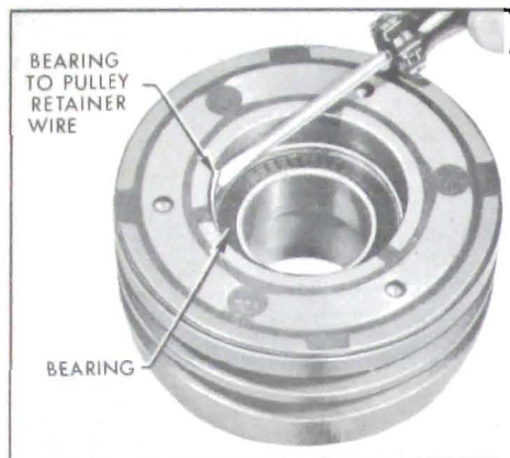
Figure 11-106—Removing Bearing to Pulley Retainer Wire
