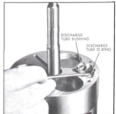
Figure 11-146—Installing Discharge Tube "O" Ring and Bushing
