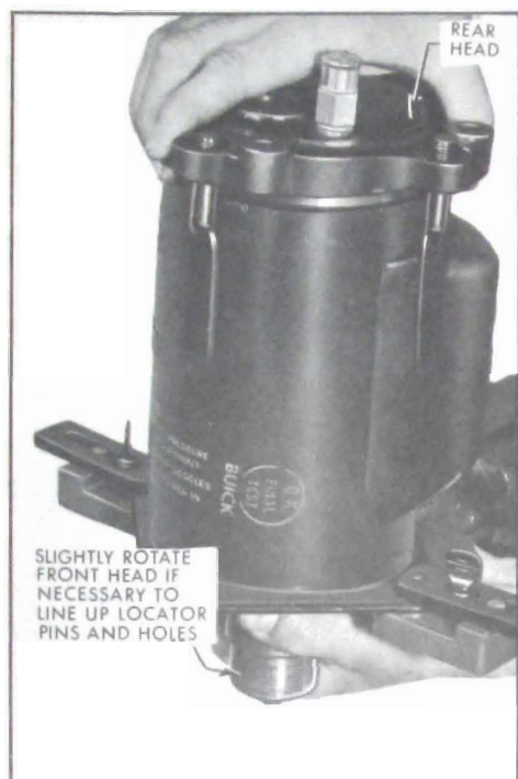
Figure 11-152—Installing Rear Head
