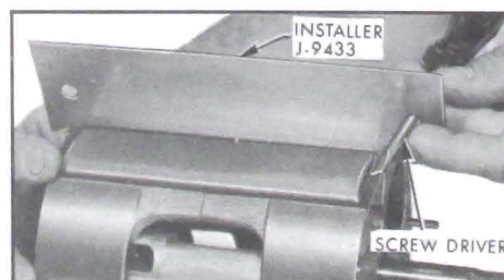
Figure 11-144—Removing Installer J-9433
