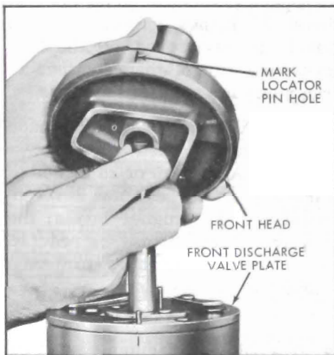
Figure 11-148—Installing Front Head on Cylinder Assembly
