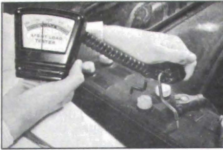
Figure 10-3—Light Load Test
