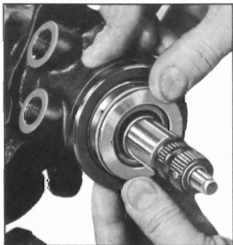
Figure 8-55—Installing Valve Assembly in Housing
