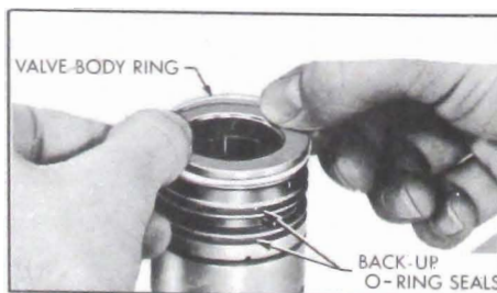
Figure 8-52—Installing Valve Body Rings
