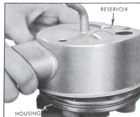
Figure 8-70—Removing Reservoir from Housing
