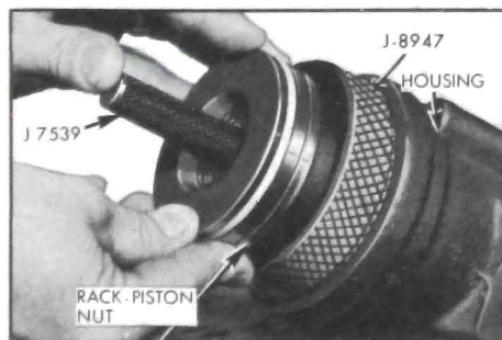
Figure 8-67—Installing Rack-Piston Nut in Housing
