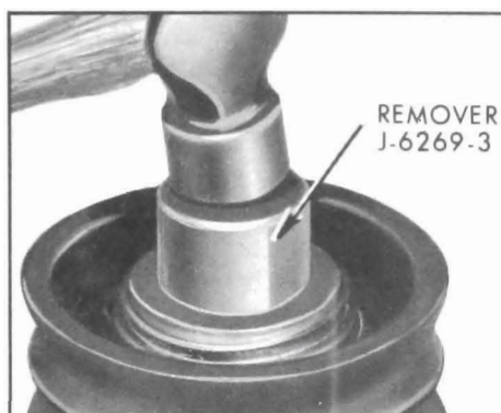
Figure 6-54—Removing Center Bearing
