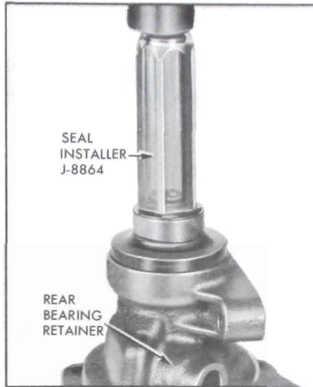
Figure 4-37—Installing Rear Bearing Retainer Oil Seal
