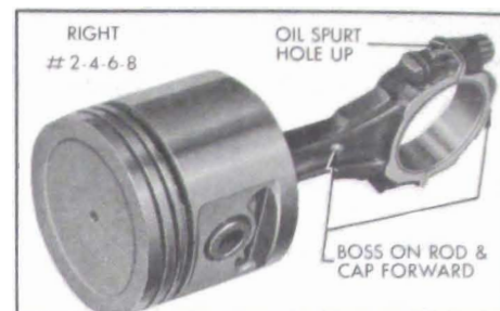
Figure 2-60—V-8 Right Bank Piston and Rod Assembly
