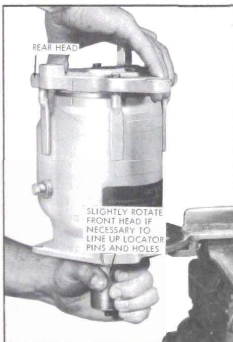
Figure 11-95—Installing Rear Head
