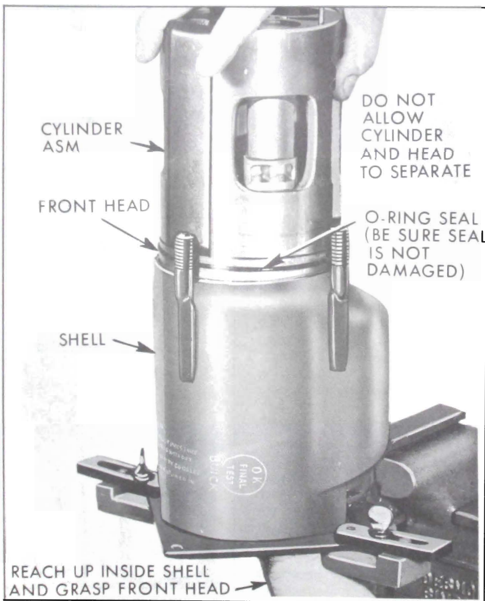
Figure 11-93—Inserting Cylinder Assembly in Shell
