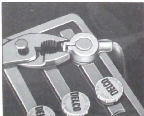
Figure 10-6—Removing Battery Cable
