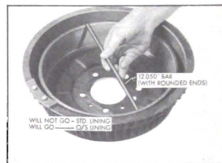
Figure 9-12—Measuring Brake Drum Size
