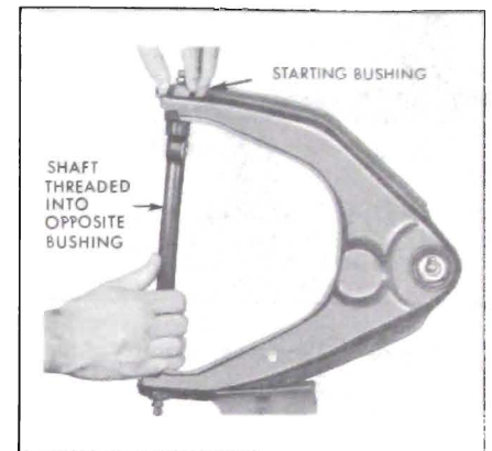
Figure 7-11—Upper Control Arm Bushing Replacement
