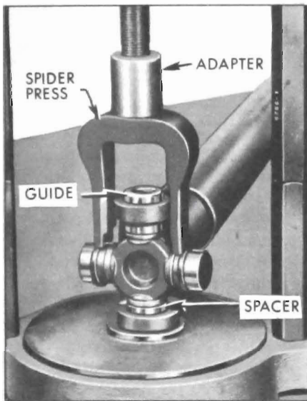
Figure 6-60—Removing Bearing with Guide and Spacer in Place
