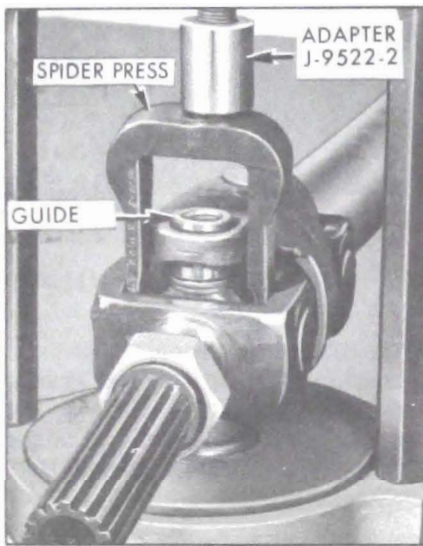
Figure 6-56—Removing Bearing with Guide and Spacer in Place
