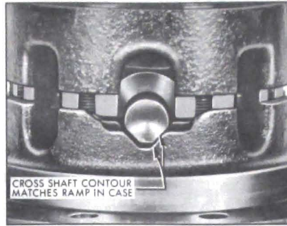
Figure 6-41—Matching Cross Shafts and Case Ramps
