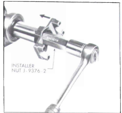
Figure 4-45—Installing Front Companion Flange
