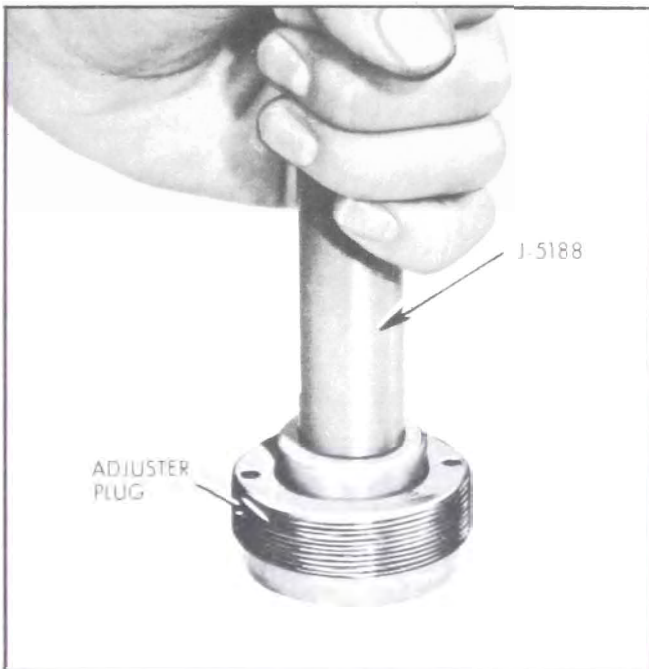
Figure 8-46—Installing Stub Shaft Seal
