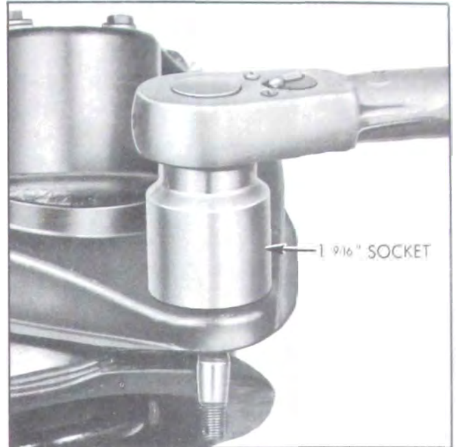
Figure 7-10—Removing Ball Joint (Upper Shown)
